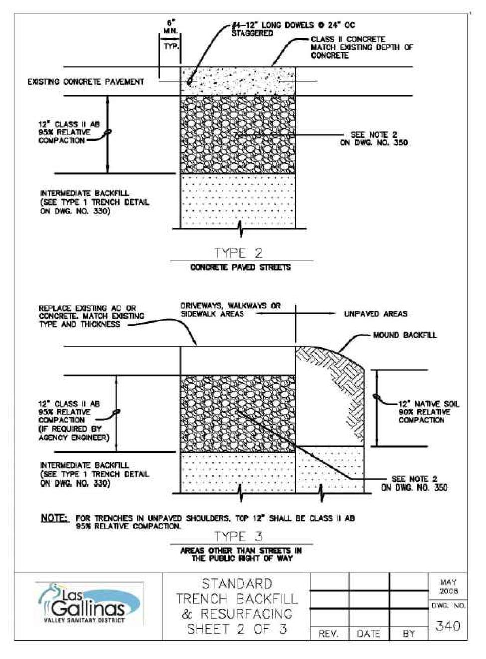
INTERMEDIATE BACKFILL SHALL BE CLASS II AGGREGATE BASE, SUITABLE NATIVE OR IMPORTED GRANULAR MATERIAL MAY BE USED IF ALLOWED BY AGENCY ENGINEER. RELATIVE COMPACTION SHALL BE AT LEAST 95%. SEE PROJECT NOTE 3
