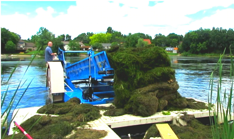
Figure 4. Eco-Cutter Aquatic Weed Harvester Unloading Collected Biomass ( https://weedersdigest.com )
