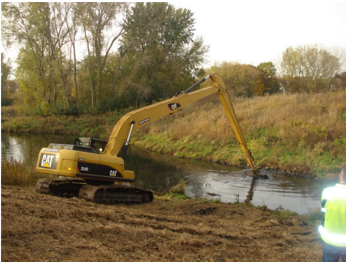
Figure 2. Long Reach Excavator
