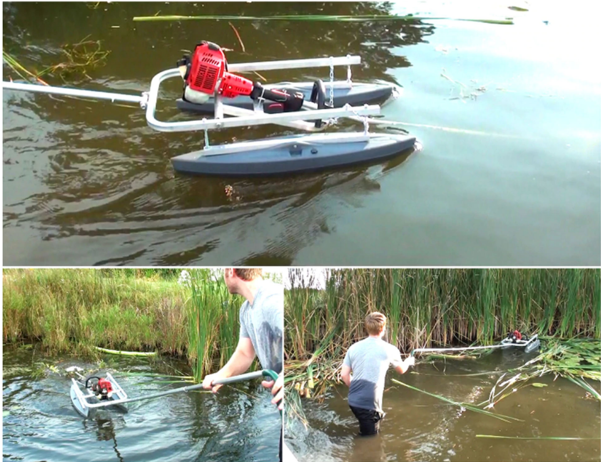
Figure 10. Aquatic Vegetation Groomer Float Attachment ( https://weedersdigest.com )
