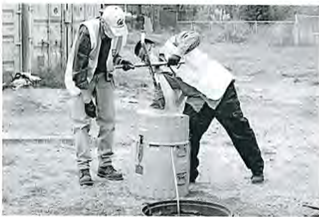
Tim Pine and Al Sanchez, employees in UC Berkeley’s Office of Environment, Health & Safety, remove a wastewater autosampler from a sewer drain, where it had been collecting samples of sewage over a 24-hour period. (UC Berkeley photo by Irene Yi)
