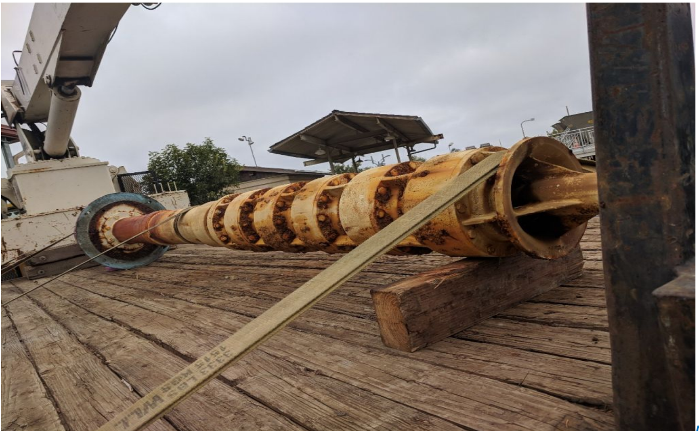
NMWD Distribution Pump Loaded for Transport to Rebuild Facility
